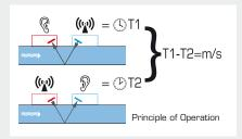
When ultrasound is transmitted between the transducers, its velocity is slightly increased when travelling in the direction of flow, and slightly reduced when travelling against the flow. The resulting transit time difference is directly proportional to the velocity of the flow in the pipe. Having measured the flow velocity and knowing the pipe cross-sectional area, the volumetric flow can be easily calculated.
