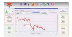
The logged instantaneous variables relevant to the main meter, and so to the whole electrical installation, can be analysed on a daily, monthly or annual basis.
