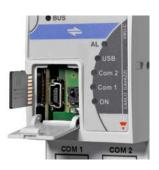
Since plant data is very important, the VMU-C EM also provides a specific micro SD slot to host, up to 16GB back-up memory. The following functions are also available:
