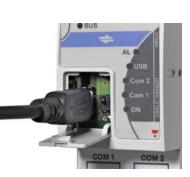
The mini USB device can be connected to a PC to perform a firmware upgrade and other service functions.
